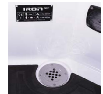
Self drainers at each side of the cockpit
