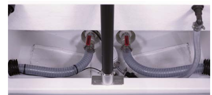
The cockpit self-draining, with check valves at the bottom inside of the transom. The automatic bilge pump is placed between the check valves and outflows in the engine well, in the upper right corner of the picture.
