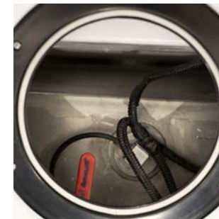
Fuel tank of stainless steel, reachable from the inspection hatch in front of the sofa.
