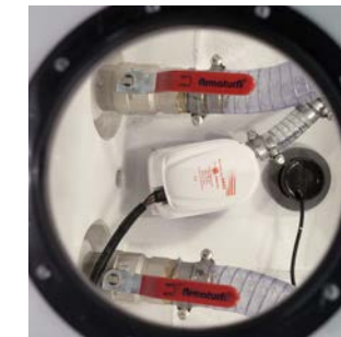
The self-draining check valves is reachable from the inspection hatch in the engine well.
